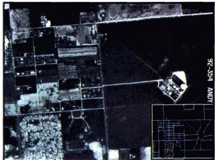
Fig. 6. In order to geo-rectify each photo, the software provides a window (upper left) in which known ground truth can be displayed. In this example, the street network is shown. Note that the areas in each display are similar. Selection of a
