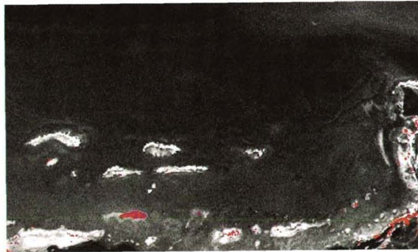
Plate 3. 1985–1989 TM Multispectral Change Magnitude image of sectors 7 and 8 with change information superimposed onto the 1985 band 1 data. Red indicates threshold magnitude increases in bands 1, 2, and 3 (sector 8). Magenta indicates threshold magnitude increases in bands 1 and 2 (sector 7). Date 1: 02 February 1985 Projection: UTM with 25-metre grid Date 2: 04 January 1989 Approximate Scale: 1:75,000
