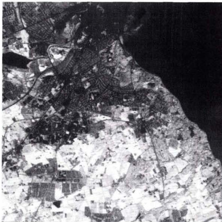
Figure 1. Test scene. 500 by 500 pixels raw IR-band of multispectral SPOT satellite image covering region just south of the city of Aarhus, Denmark. (© SPOT Image 1988 CNES.)
