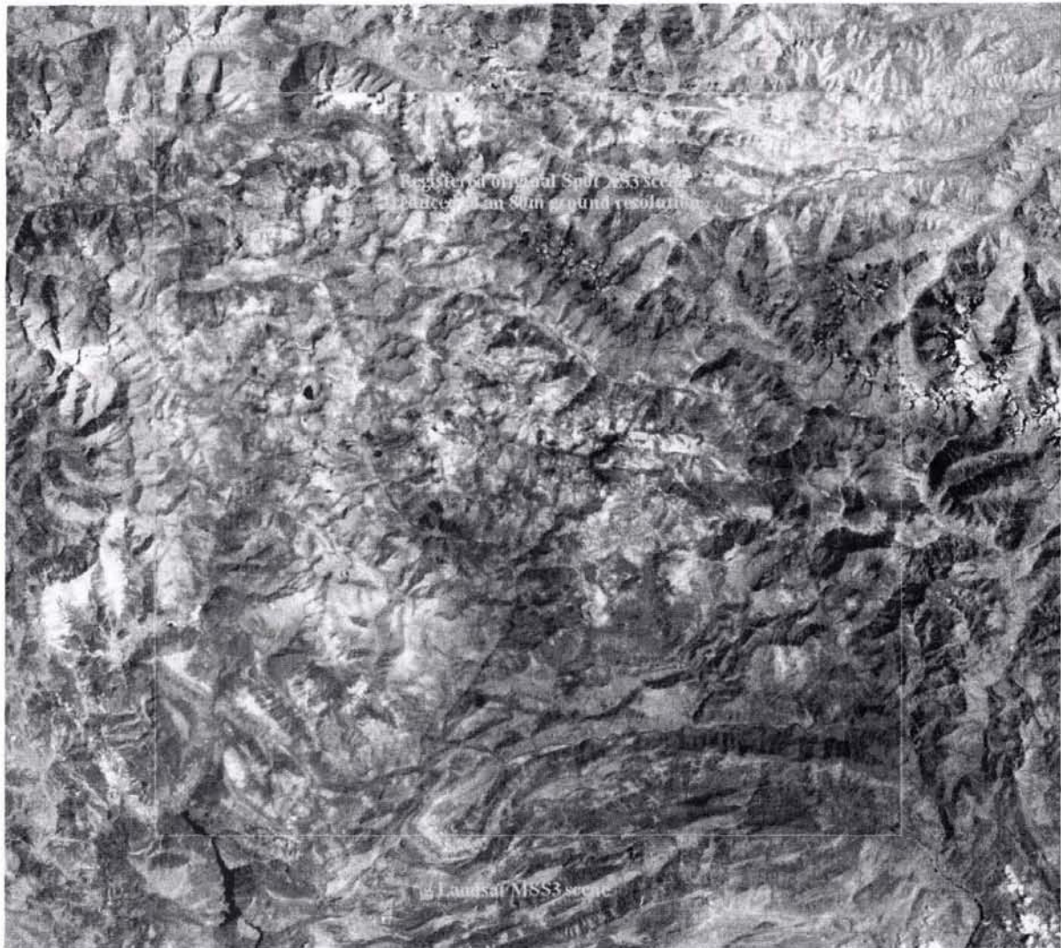
Figure 8. The original registered SPOT image, reduced to an 80-m ground resolution and enlayed into the MSS scene.
