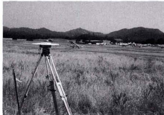
Figure 3. Aircraft taking off, with GPS reference station in the foreground.
