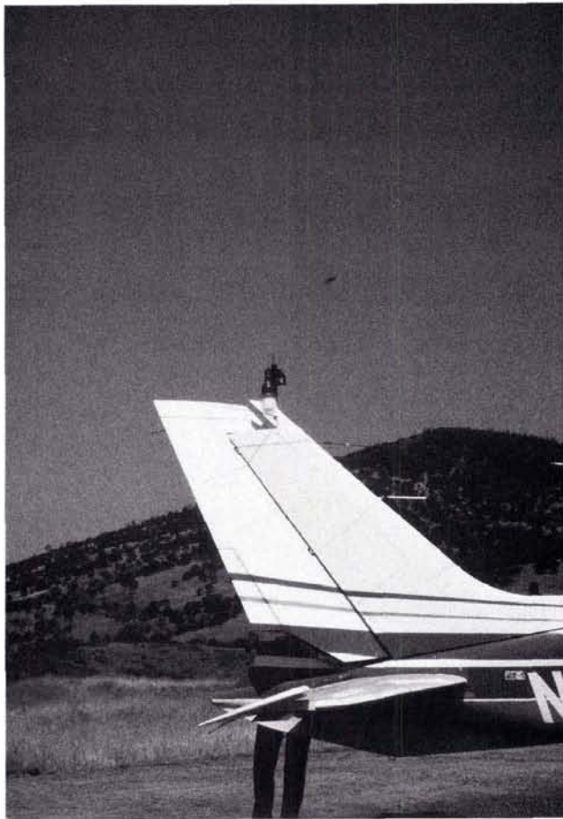
Figure 1. GPS Antenna mounted on tail of aircraft.
