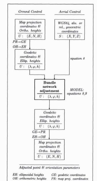
Figure 3. Sequence of coordinate transformations for Equation 8 model.
