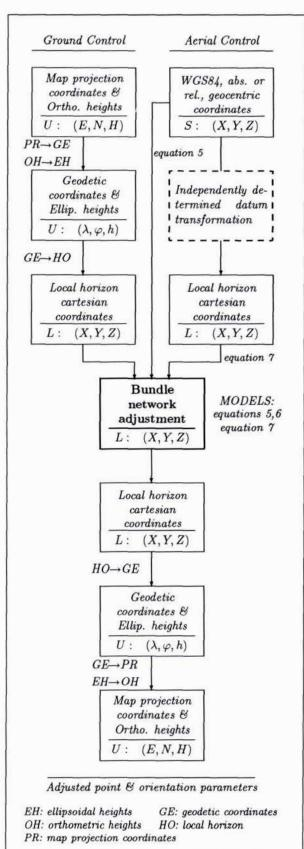
Figure 2. Sequence of coordinate transformations for Equations 5 and 7 models.
