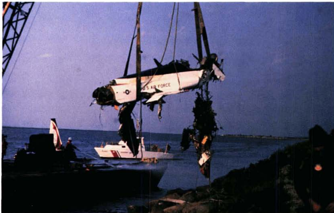
Figure 1. The lead Air Force demonstration team pilot was killed in this 1981 accident when his T-38 struck a gull on takeoff during a practice session.
