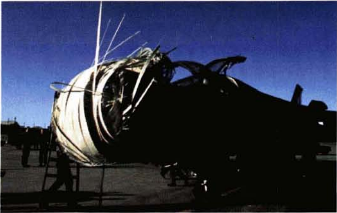
Figure 2. This USAF F-111 struck a Red-tailed Hawk on a low-level training mission in New Mexico.
