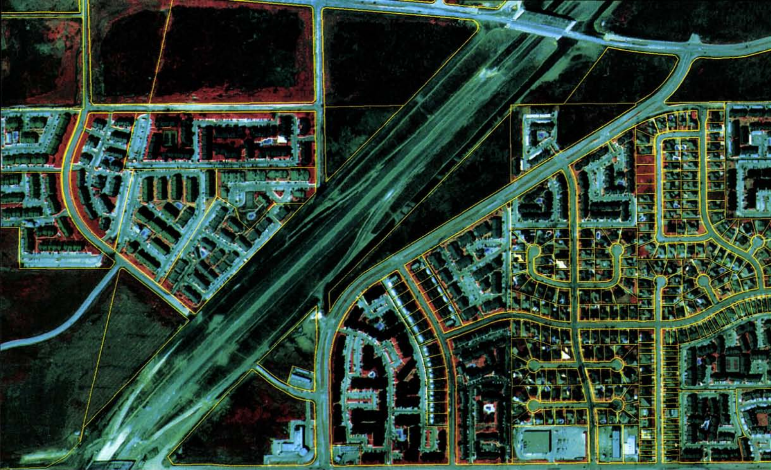
Figure 1. A Subset Composed of Approximately 20 ADAR System 5000 Scenes (In Color Infrared: RGB Display Showing Near IR, Red, and Green Spectral Bands, Respectively) Including a Vector Overlay of Property Parcel Data.
