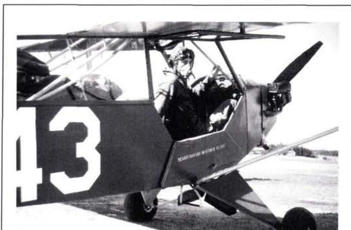
Figure 1. The Cub offers low stall speed and excellent visibility. A microphone built into the face mask enables the photographer to communicate with the pilot while the window/door is open.
