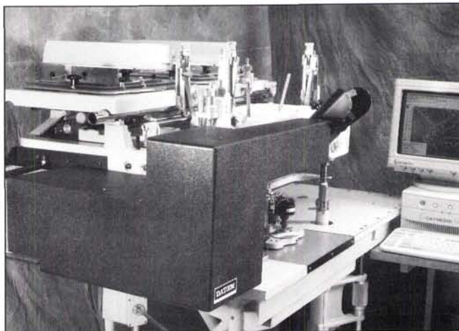
The S/I shrouding helps maintain the intensity of the internal monitor. The hardware and covers are adapted to each application.
