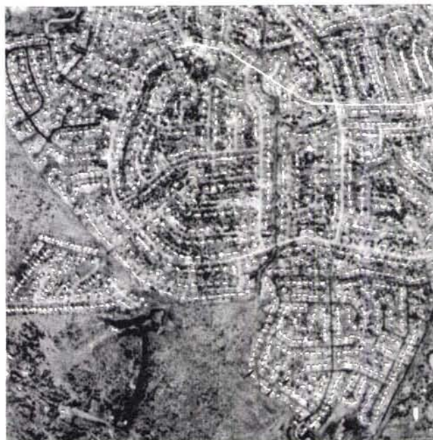
Figure 2. Individual dwelling units were extracted from the high spatial resolution CAMS 5- by 5-m data using band ratioing techniques. The house pixels were then "clumped" and converted into polygons for comparison with 1990 Bureau of the Census block group housing statistics.
