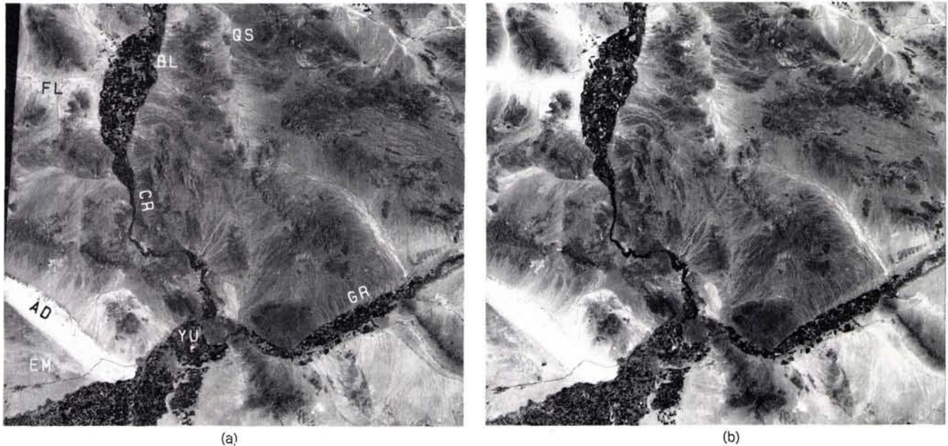
Figure 1. Full-scene, calibrated Landsat MSS band 5 (red spectral band) image acquired on 4 April 1992 (a) and 1 July 1992 (b). They have been geometrically and radiometrically calibrated so that the same DN represents the same ground reflectance. For comparison, the same contrast stretch has been applied to each image. EM, East Mesa; AD, Algodones Dunes; YU, Yuma; GR, Gila River; CR, Colorado River; FL, Ford Dry Lake; BL, Blythe; and QS, Quartzsite.
