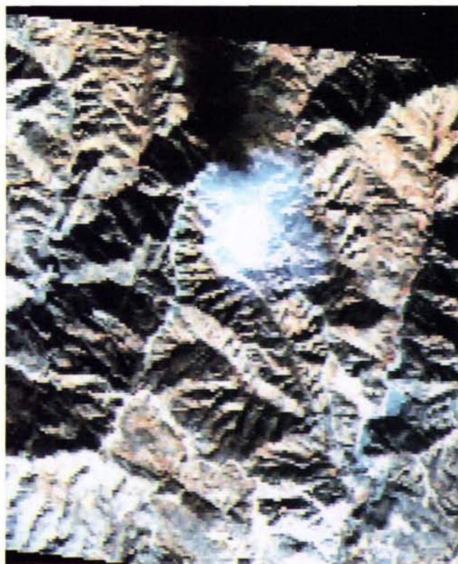
Plate 1. Visible light (4,3,2) image of the Lodi Canyon fire at 2000 GMT, 12 December 1986, contrasted with a false-colored single-band image from the infrared (band 10). Images are from the Daedalus Thematic Mapper Simulator, with a ground resolution of 25 metres.
