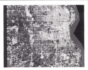
Figure 9. Final classification of the Milwaukee, TIGERbased PCA data set. White delineates high-density urban land cover, while the medium-gray and dark-gray toned areas represent medium and low-density urban land cover, respectively.
