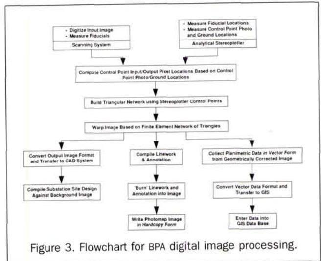
Figure 3. Flowchart for BPA digital image processing.
