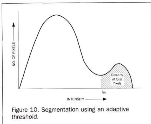
Figure 10. Segmentation using an adaptive threshold.
