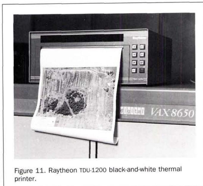
Figure 11. Raytheon TDU-1200 black-and-white thermal printer.
