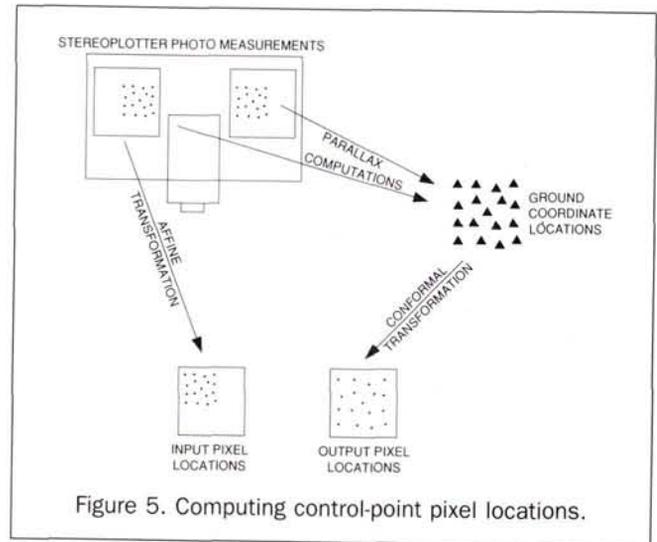
Figure 5. Computing control-point pixel locations.
