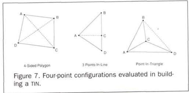
Figure 7. Four-point configurations evaluated in building a TIN.
