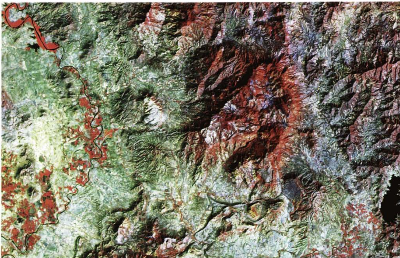
Plate 1. Landsat Thematic Mapper (TM) color composite image (Bands 7, 3, and 4 as blue, green, and red, respectively) of northern Guerrero between Ciudad Altamirano and Nuevo Copaltepec taken on 25 January 1986. The image is the same scale as the geologic map in Figure 2. The body of water in the lower right is the Presa Vicente Guerrero reservoir.
