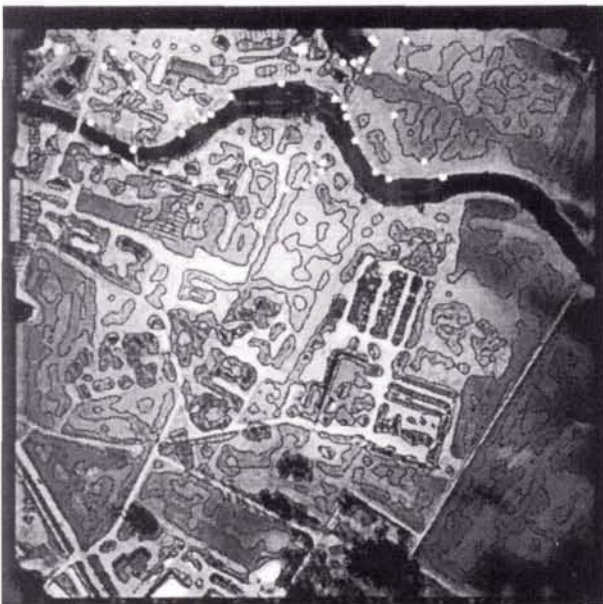
Figure 7. Two images of neighboring strips were matched. Despite a shift between the two strips and the marginal sidelap, many correct matches were found.
