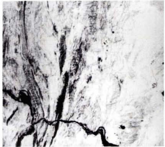
Figure 9. Brightness saturation on original Level-2 OPS Channel 8. Simultaneous observation of geological details in both dark or brightly saturated areas is impossible.
