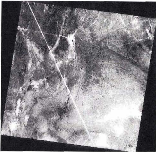
Figure 6. Vegetation fraction of the study area, Long Valley, Nevada. With sagebrush spectrum as a vegetation endmember. Calculated vegetation fractions range from 0.24 to 0.38. The image is produced by scaling the fraction values 0 to 255. Dark tone is less and brighter tone is more vegetation.
