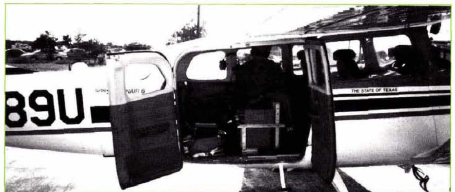
FIGURE 4. An Optech ALTM-1020 airborne laser terrain mapping system was installed in this single-engine Cessna 206 to map over 163 sq. km in one day over Galveston Island and Bolivar Peninsula.
