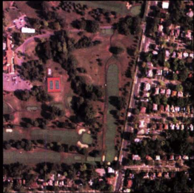
FIGURE 2. 800 pixel x 800 pixel portion of a digital orthoimage with simulated 1-m collection and 0.6-m product GSD. The display scale and extent are the same as in Figure 1.
