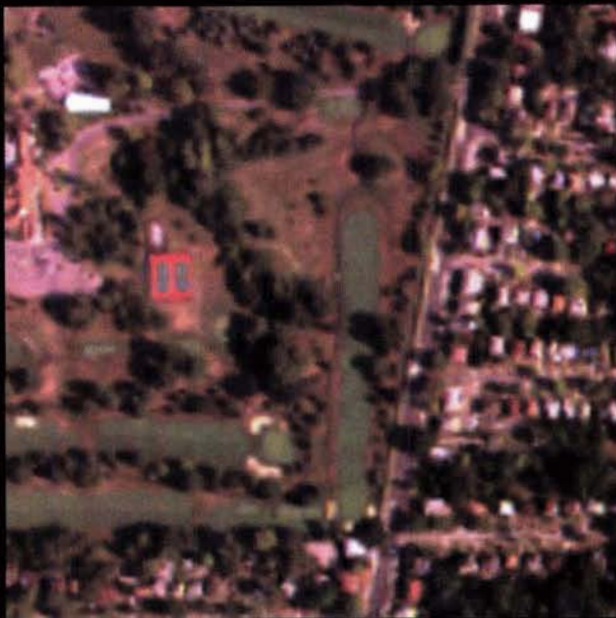
FIGURE 3. 800 pixel x 800 pixel portion of a digital orthoimage with simulated 3-m collection and 0.6-m product GSD. The display scale and extent are the same as in Figure 1.
