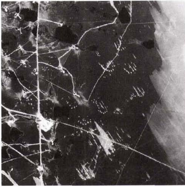
Figure 4. Postwar SPOT panchromatic image (25 March 1992) of a section of the Burgan oil field showing the dark "tarcrete" from the oil well fires. Bright lines are roads that were built by fire-fighting crews, and black spots are oil lakes. Pits and sand trenches dug by fire-fighting crews appear as bright dots. Image covers an area of 10 by 10 km. See Figure 1b for location.
