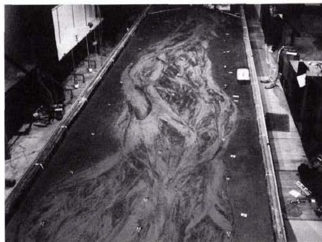
Figure 1. Oblique photograph of the experimental flume with small-scale river model.
