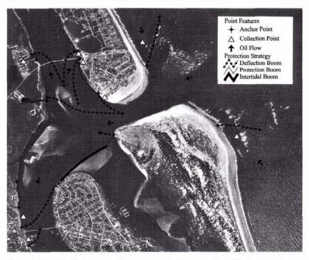
Figure 2. The tidal inlet protection strategy for St. Augustine, Florida, depicts anticipated oil flow directions, boom anchor points, collection points, and boom placement strategies. The information is overlaid on rectified black-and-white vertical orthophotography.
