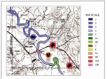
Plate 2. A River Reach Sensitivity Index (RSI) map for a section of the Leaf River, Mississippi. PB refers to a point bar which is an ideal oil collection location. The numbers beneath the icons represent resources-at-risk summarized in the database (refer to Table 5 for an example).
