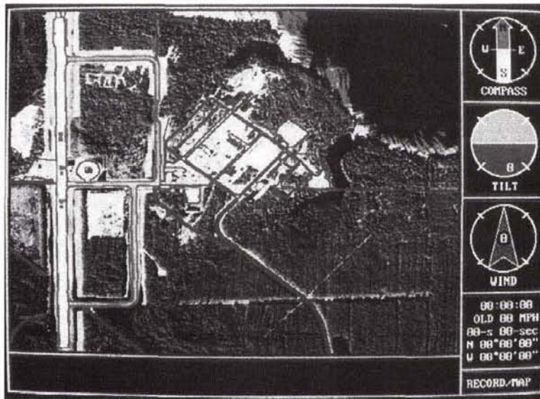
Figure 2. The moving map as integrated into VAPERS and displayed on the LCD screen.
