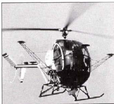
FIGURE 2. GPS Equipped helicopter used to collect laser imagery and videos for the Long Island Rail Road.
