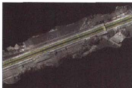
FIGURE 3. Planimetric view of laser imagery for Smithtown train station, with a vectorized track centerline.
