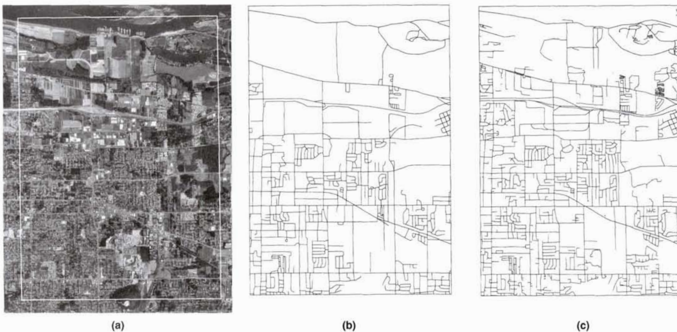
Figure 5. (a) DOQ of Camas, Oregon (SW quadrant). The white rectangle delineates the area used for DOQ/DLG comparison. DLG roads (b) and roads digitized from DOQs (c) for Camas, Oregon (SW quadrant). Note the increase in roads due to recent development on the DOQ.
