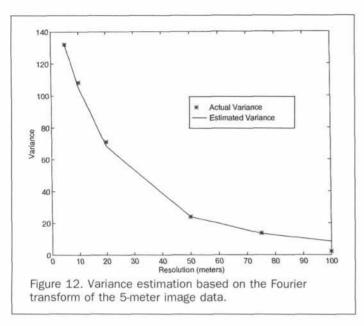
obtained at 30 meters could be expected. This is apparently due to the relatively large size of objects in this scene, and the large range of the observed variogram. Because the nugget effect of the target sensors is not included, the plotted values represent what the variance of such a scene would be in the absence of sensor noise.
