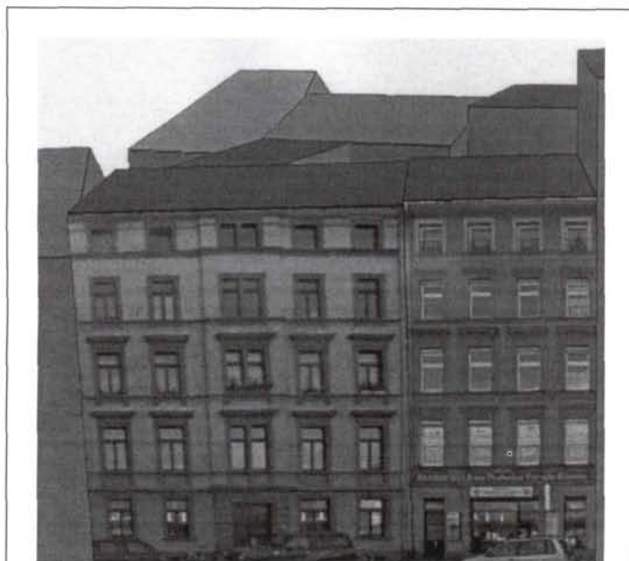
Figure 17. Faces mapped to corresponding 3D surfaces.
