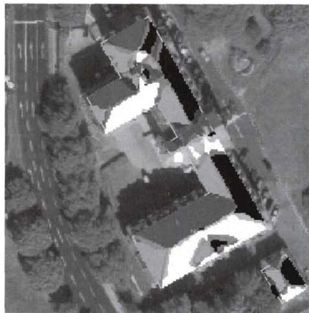
Figure 8. The original ground plan and segmented roof regions.
