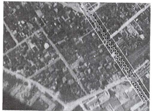
Figure 21. Third experimental field and the extracted road's feature points using EPIS at a 5-pixel EPI interval.
