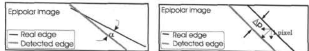
Figure 29. Detected and real edge. (a) The trajectory deviates from ideal direction. (b) The trajectory shifts along the u and v axes.
