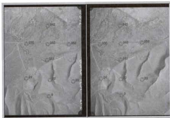
RMS (m) at 9 Check Points, Using 6 Control Points, (Bishop, 1:6000)
