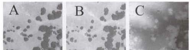
Figure 6. A stereo pair of oak wood land and its disparity map. A: left image. B: right image. C: the disparity map referenced to the left image.
